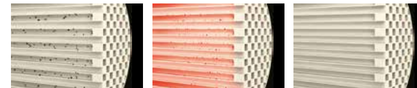
1. Particulate matter trapped 2. Regeneration starts 3. Regeneration completes*
