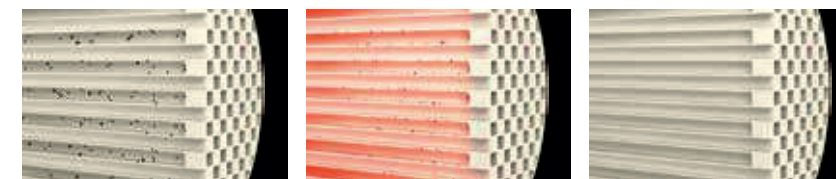
1. Particulate matter trapped 2. Regeneration starts 3. Regeneration completes*
